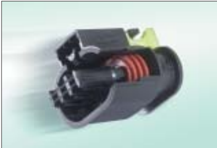
Ignition connector. The ignition connector is mounted on top of the engine. Stanyl was chosen here for its heat stability in combination with its mechanical performance and chemical resistance.
