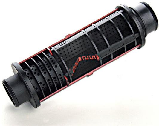
A wide-band resonator from Woco Motor Acoustic Systems USA Inc. won top honours in the Society of Plastics Engineers Automotive Division "Most Innovative Use of Plastics" Award's powertrain category. Made with DuPont™ Zytel® nylon 66 due to the material's unique combination of mechanical and thermal properties, the resonator silences "turbo-whine", eliminates insulation material and improves durability by integrating injection moulded high and low frequency parts into a single assembly.
