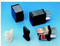
Relay for automotive electrical systems meets needs for reliability and low cost. Assembly is fully automated and requires no fasteners. Materials: Bobbin, Rynite® 530 PET thermoplastic polyester resin; base and cover, Crastin® SK605. Manufacturer: Saturn Electronics and Engineering Inc., Auburn Hills, Michigan, USA.
