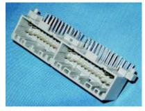
For this connector used in an automotive power seat control module, Thermx® PCT high performance polyester provided a drop-in replacement for PBT. This allowed a shift to reflow solder assembly without building a new mold. Material: Thermx® CGT33. Manufacturer: Tyco Electronics, Greensboro, North Carolina, USA.
