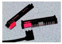
This power distribution connector relies on Zytel® HTN to meet demanding requirements. They include high-temperature resistance for solder assembly, robust mechanical properties and surface hardness to allow for press-fit pin configurations, dimensional stability and good molding productivity. Material: Zytel® HTNFR52G45BL. Manufacturer: FCI, Etters, Pennsylvania, USA.
