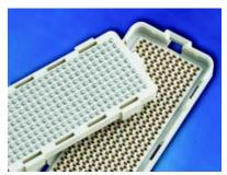
Innovative high-density connector system relies on precision molding capability, dimensional stability, high-temperature resistance and reduced thermal expansion coefficient of a special Zenite® LCP liquid crystal polymer resin. Material: Zenite® 3226L. Manufacturer: FCI, Etters, Pennsylvania, USA.
