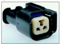
In a two-way connector for an automotive fuel injector, Zytel® DMX modified nylon fulfills needs for consistent mechanical properties and dimensions under varying humidity conditions. Material: Zytel® DMX65G15H. Manufacturer: Molex Corporation, Auburn Hills, Michigan, USA.
