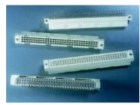
In these DIN 41612 connectors, the excellent flow properties of a glass-reinforced Crastin® PBT thermoplastic polyester resin are crucial for filling intricate details with wall sections as thin as 0.012 in. (0.3 mm). Material: Crastin® SK655FR1, a UL94 V-0 resin. Manufacturer: ERNI Components, Adelberg, Germany.
