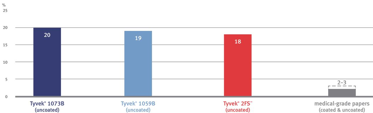
**Figure 7. Elongation (MD) properties of DuPont™ Tyvek® styles and medical-grade papers (ASTM D5035 and EN ISO 1924-2 @ sample length of 5 in. [13 cm] and rate of extension [ROE] of 2 in./min [5 cm/min]).**
