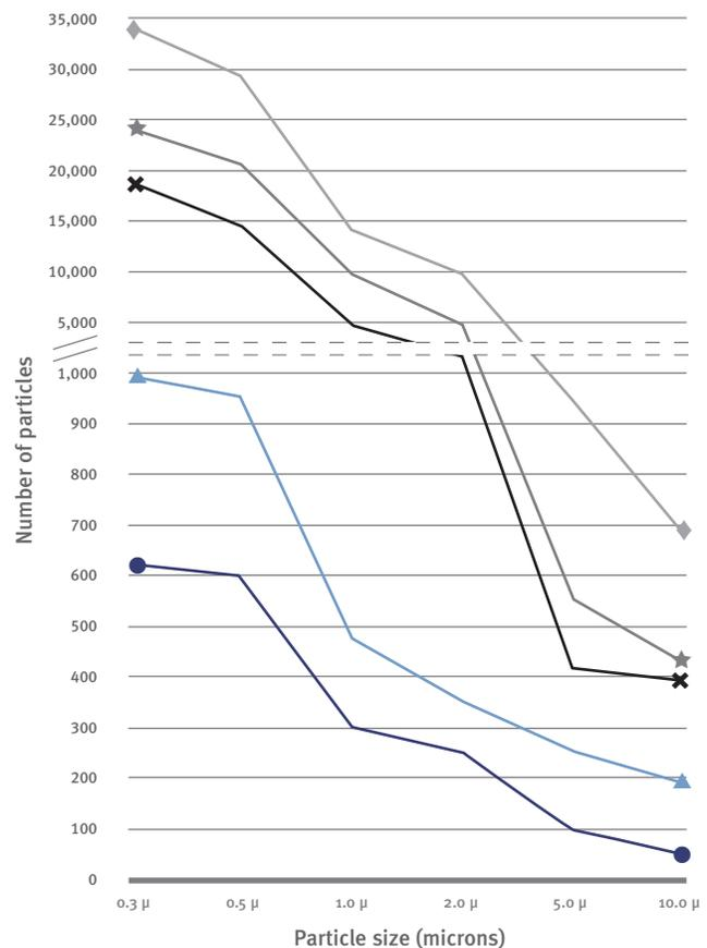
**Figure 9. Particle generation properties of DuPont™ Tyvek® styles and medical-grade papers (as tested by an internal DuPont protocol).**
