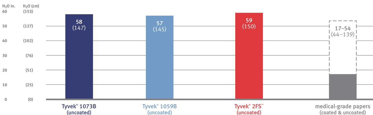
**Figure 8. Hydrostatic head properties of DuPont™ Tyvek® styles and medical-grade papers (AATCC TM 127 and EN 20811 @ rate of use of 60 cm H<sub>2</sub>O/min).**
