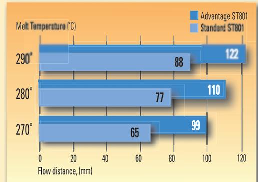
Test conditions: Snake mold with 1 mm channel depth; injection pressure 80 MPa (11,500 psi), injection speed 50 mm/sec; mold temp., 70°C; moisture, 0.1%.
