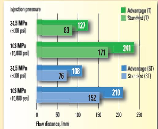
Test conditions: Snake mold with 1 mm channel depth; melt temperature, 290°C (555°F); injection speed 50 mm/s; mold temperature, 70°C (160°F).
