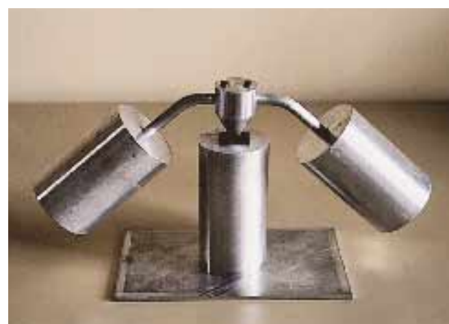
Fig. 1. Hot ball pressure test apparatus
