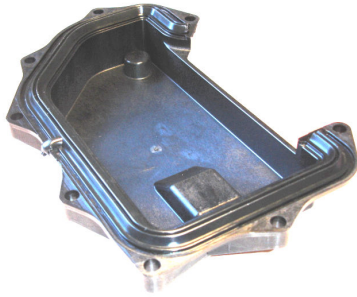
Fig.1 AUTO/Oil system application of a structural cover moulded in Zytel® 70G50HSLA BK039B featuring very high stiffness and excellent surface finish integrating a fast curing thermoset gasket in DuPont™ VAMAC®.
