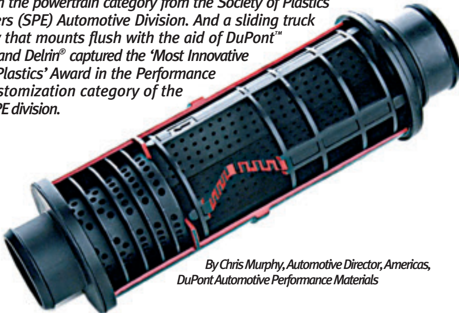
The turbo resonator, developed by Woco Motor Acoustics using Zytel®, eliminates insulation materials by integrating high- and low-frequency attenuating parts into a single assembly while silencing 'turbo whine'.
