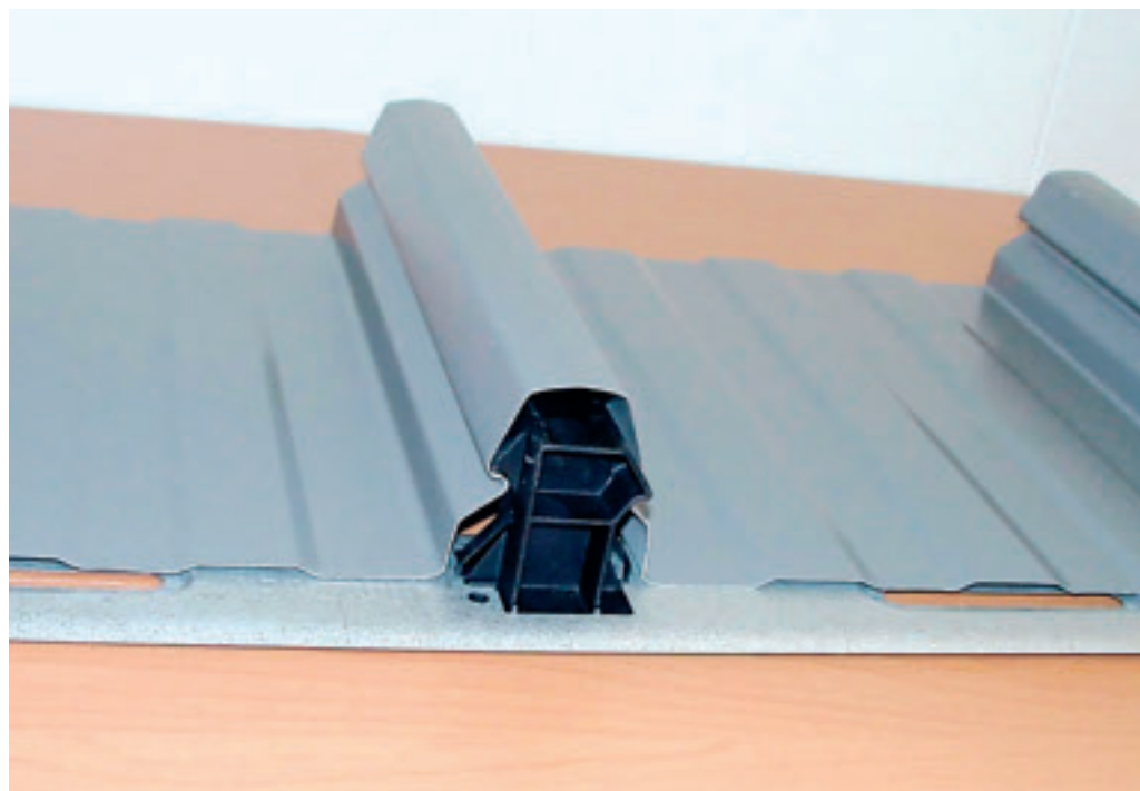
Three Zytel® clips are inserted through a steel strip the width of a single roof sheet, before the sheet itself is locked in place by pushing the pre-formed upstands in the profile onto the clips.
