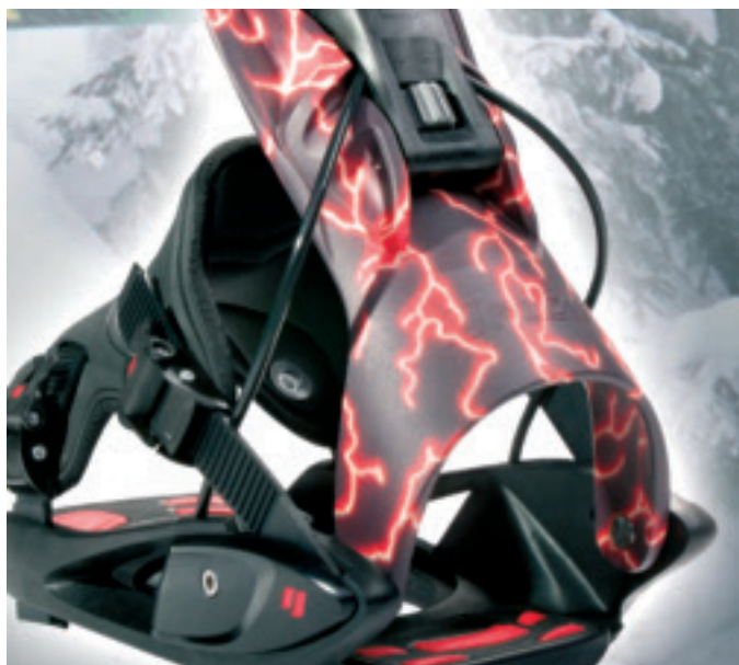
The decoration on these snow-board binding parts made of Zytel® nylon is applied by means of sublimation. The decoration is scratch- and abrasion-resistant, because, with this new technology, the inks are absorbed into the surface of the plastic.
