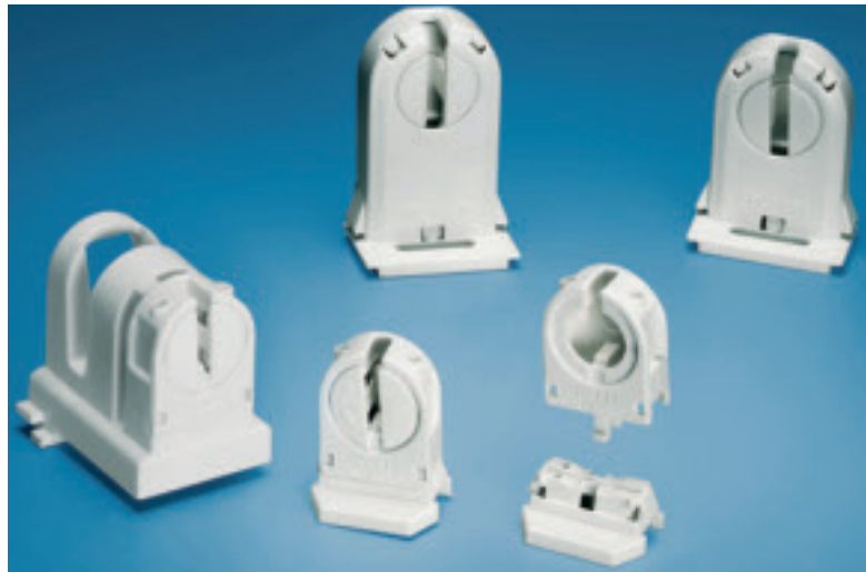
Leviton engineers took advantage of the toughness, resilience and high flow of Crastin® PBT and incorporated integral features for snap-fit assembly and lamp locking, thus eliminating metal fasteners and simplifying assembly.
