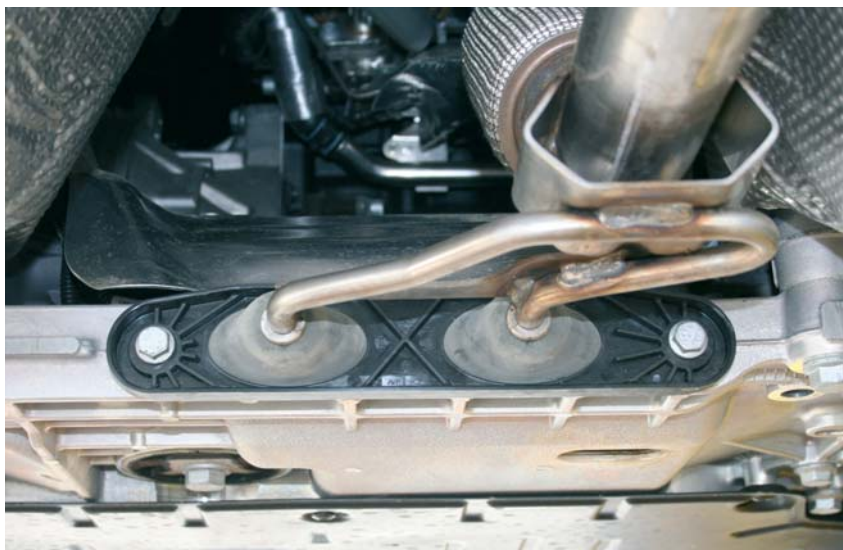
The new bracket from anvisgroup is the first polymer mounting for the 'hot end' of the exhaust module
