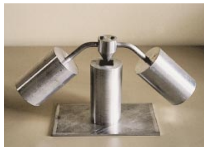
Fig. 1. Hot ball pressure test apparatus
