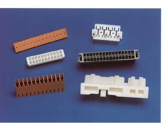
High molding productivity in FR nylon. Video connector at lower right and board-mounted connectors shown are all molded from flame-retarded grades of Zytel® nylon. In addition to meeting electrical safety requirements, the resins provide the high melt flow needed for rapid molding with complete filling of small features.
