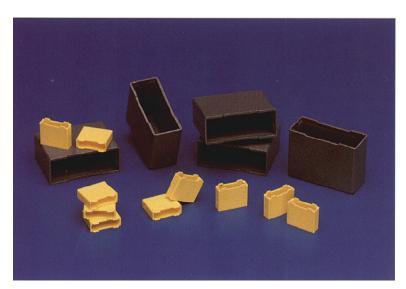
Thin-wall capacitor cases. Made with fast-molding grades of Crastin® PBT, these capacitor cases are right on target for dimensional tolerances and more. The resin also provides the required dielectric properties, resistance to board cleaning chemicals, toughness and strength. Manufacturers: yellow cases, Thomson; green cases, Rodenstain; gray cases, Arcotronics.
