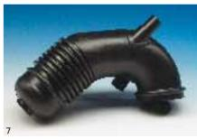
7. Another HYTREL® application in automotive components is the blow-moulded air-duct made of HYTREL® HTR4275 BK. VW has adopted this innovative technology and benefits for noise reduction, light weight and an overall reduction of the number of parts in the engine compartment, due to its multi-functionality.
