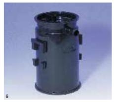
6. Carbon canisters are devices incorporated into modern vehicles, which help to minimise fuel emission levels. They are often located low down in the engine compartment, being exposed to flying road surface debris, high temperatures, oil and fuel vapour. Tennex (UK) have chosen to produce a canister housing and lid in ZYTEL® ST which readily resists this highly demanding environment and provides an excellent barrier to fuel vapour.
