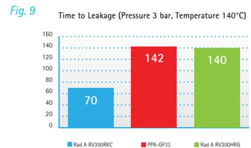
*In a leakage test with a vibration welded tank cover, Radilon® A RV300HRG exhibits the same behaviour as polyphthalamide (PPA), which is usually recommended for use in contact with engine cooling liquids.*
