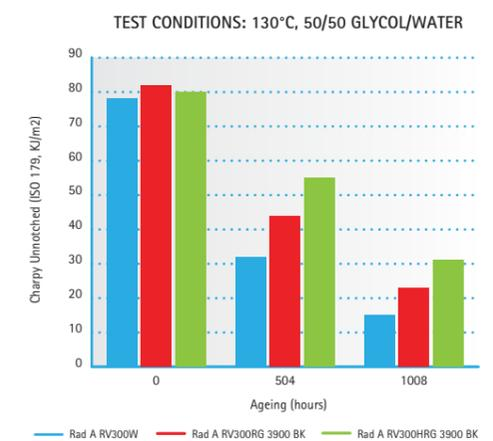
As we can see from Fig. 3, in the case of Radilon® A RV300HRG, the time to Charpy unnotched impact half life in a glycol/water mix at 130°C is:
