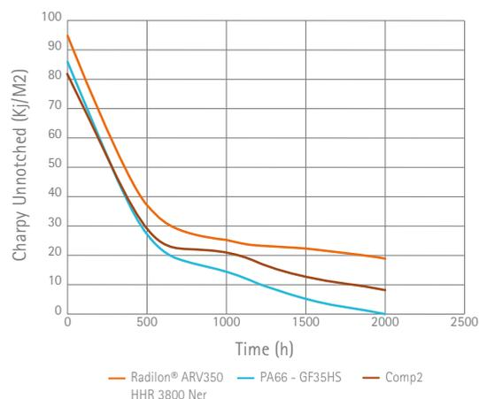
**FIG.4 - HEAT AGEING IN AIR AT 210°C**
