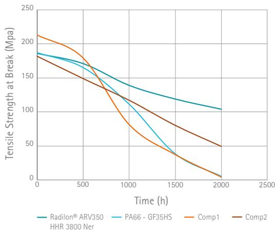
**FIG.3 - HEAT AGEING IN AIR AT 210°C**
