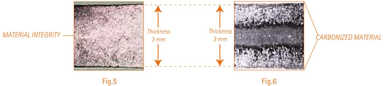
As we can observe from the cross-section in Fig.5, after 1000 hours of heat ageing at 210°C, the Radilon® A RV350 HHR specimen has remained practically intact, except for slight degradation on the surface. In contrast, as we see in Fig.6, the heat stabilized PA66-GF35 specimen exhibits a deeply degraded structure after the same heat ageing process: about 70% of the specimen thickness is destroyed.
