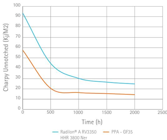
After 2000 hours of heat ageing in air at 200°C, Radilon® A RV350 HHR 3800 Ner (High Heat Resistance) exhibits Charpy unnotched impact strength degradation comparable to polyphthalamide (PPA):
