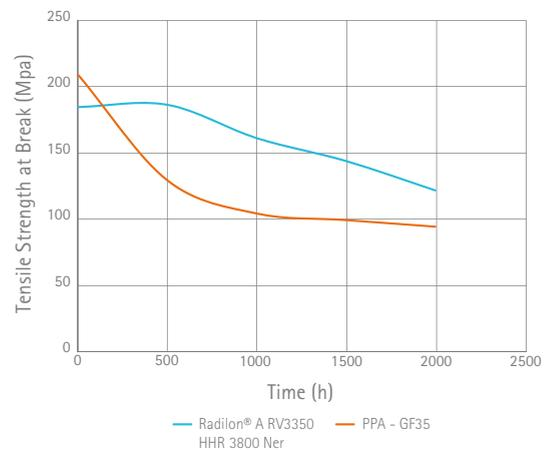
After 2000 hours of heat ageing in air at 200°C, Radilon® A RV350 HHR 3800 Ner (High Heat Resistance) exhibits less tensile strength at break degradation than polyphthalamide (PPA):
